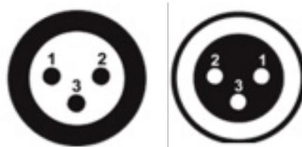
The termination is prepared by soldering a 120Ω resistor between pins 2 and 3.
